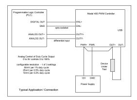
Once power is applied to the PWMC 400, the unit will operate as configured (analog or USB to PWM duty cycle out).
