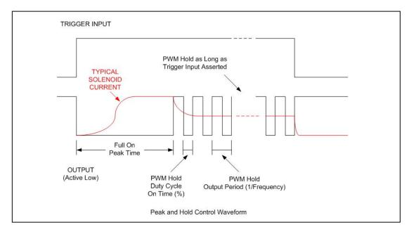
The Model 500 PWM Peak and Hold PWM Controller has two rotary switches on the face of the unit which allow for precise setting of the peak time and the hold PWM duty cycle. Timing and PWM control are generated using microcomputer circuitry internal to the Model 500 unit. Refer to the figure and tables below to set the Model 500 peak time and hold PWM duty cycle.
