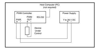
Refer to the User's Manual for other possible connection configurations (Section 3.0 Installation).
